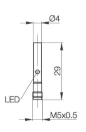
Inductive Sensors BES G04EC-POC15B-S26G D4 x 29 normally-closed Sn=1,5mm shielded
